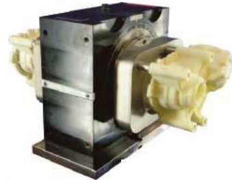
Multi-side machining of plastic parts with double clamping
