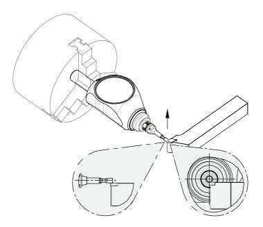
**5** Probing (Z axis) (Determine tool length)
